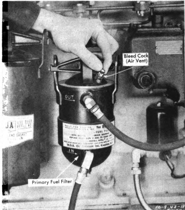
Figure 27. Removing the Air Vent in the Primary Fuel Filter
