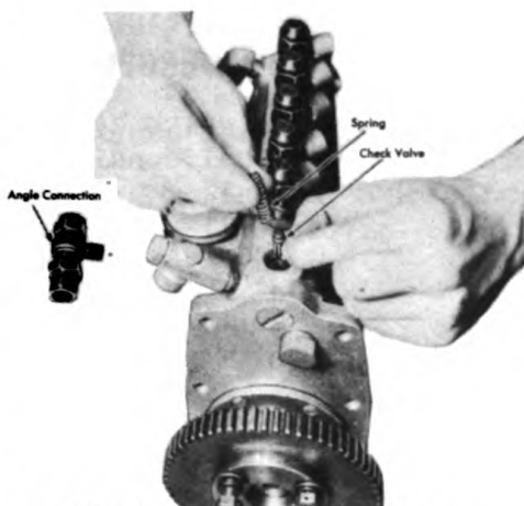
Figure 326. Removing Check Valve.
