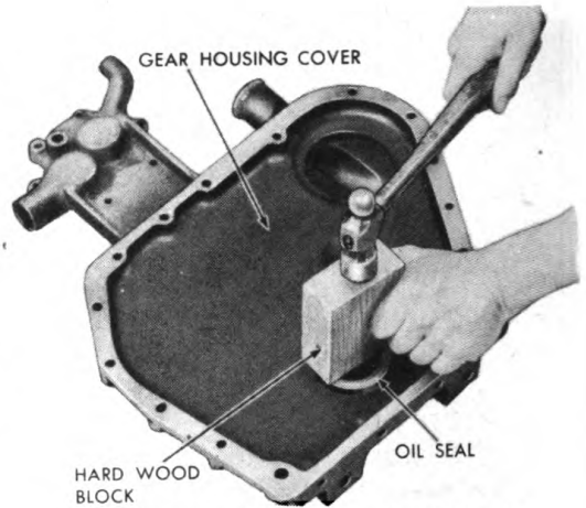
Figure 194. Installing Oil Seal.
