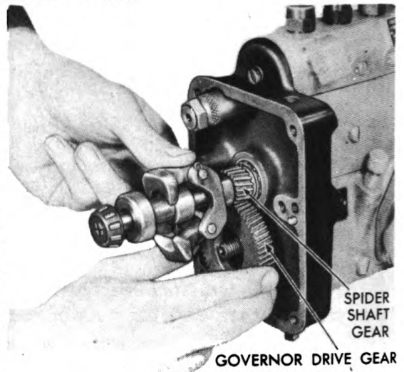
Figure 223. Installing Governor Drive Gear and Spider.
