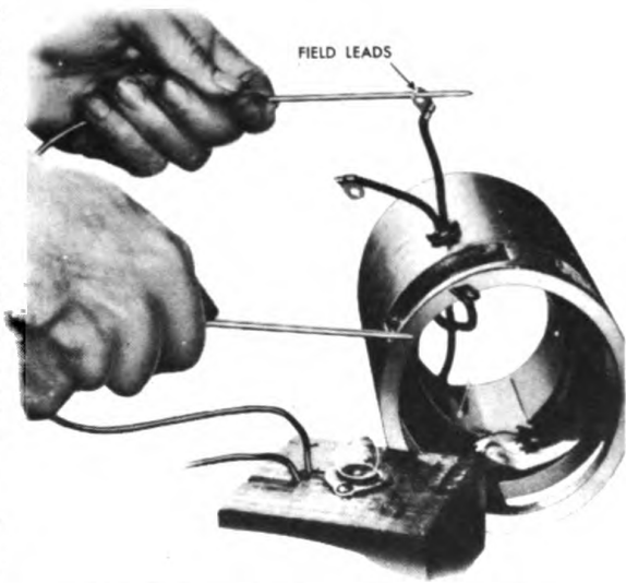
Figure 240. Testing Field Coils for Grounds.
