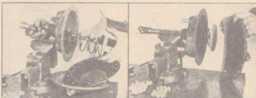
FIGURE B. BRAKE CHAMBER—REPLACING SPRING
