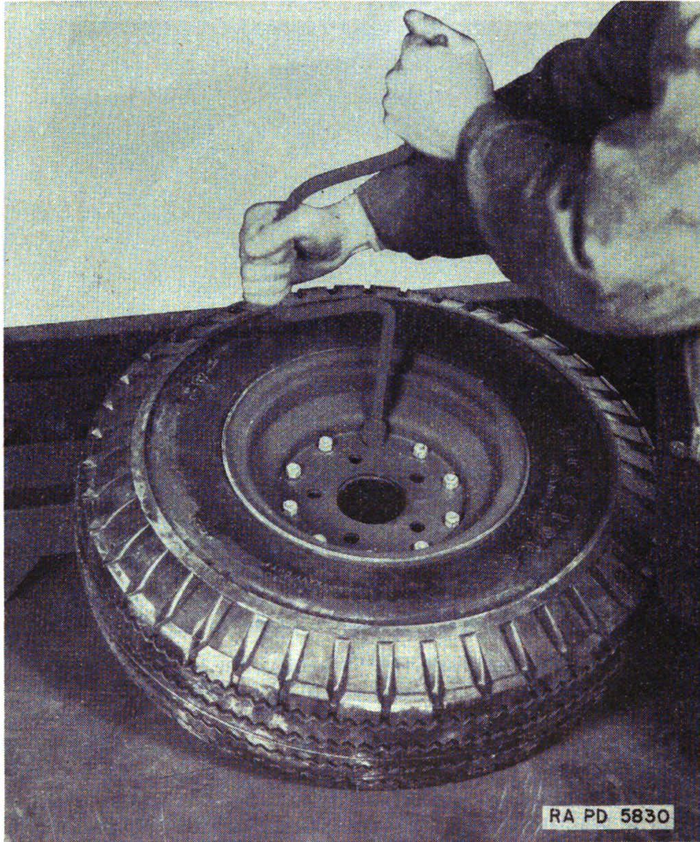
FIGURE 17.—Front wheel disassembly.
