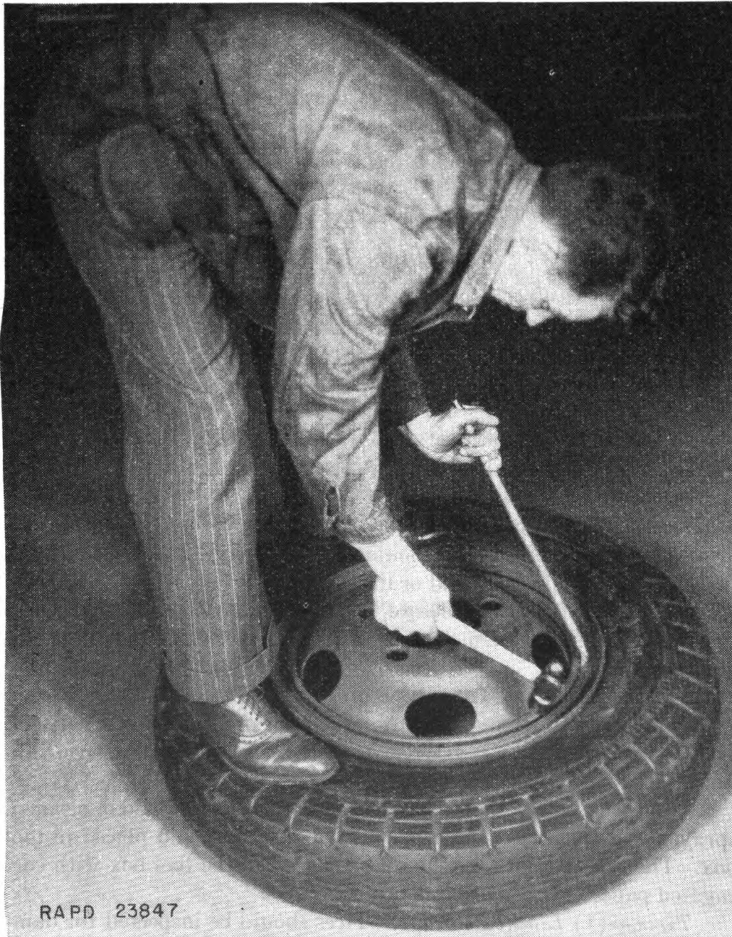
FIGURE 20.—Installing side ring.
