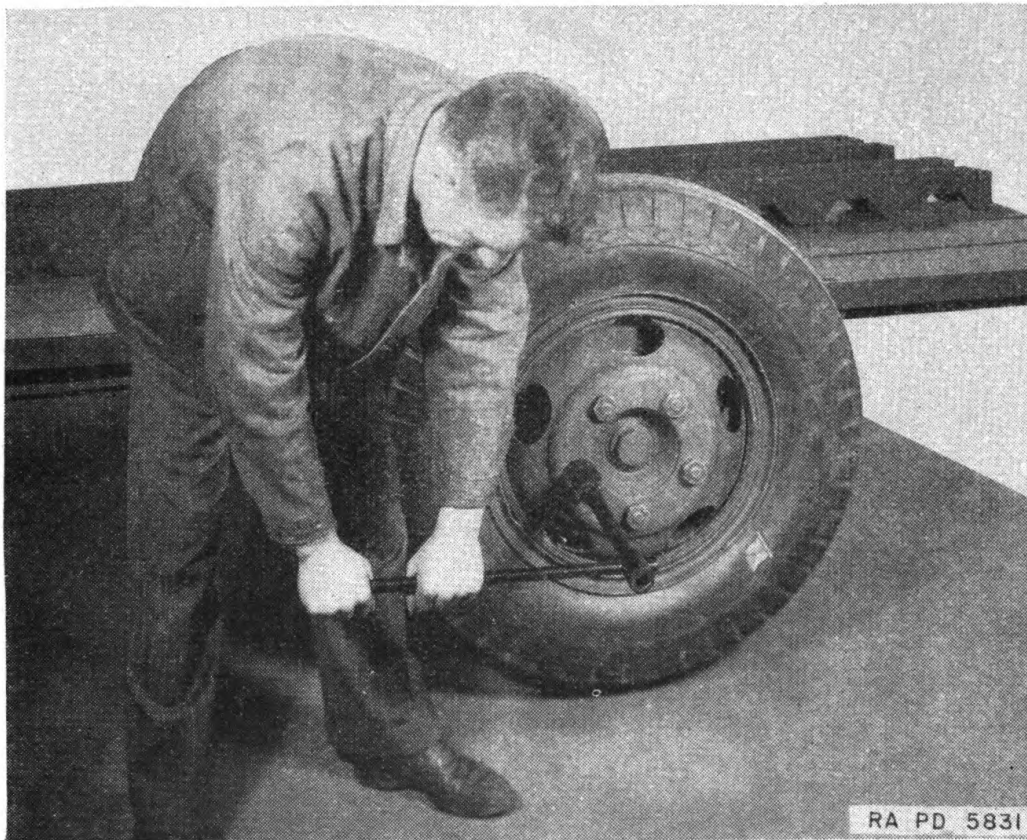
FIGURE 18.—Rear wheel removal.
