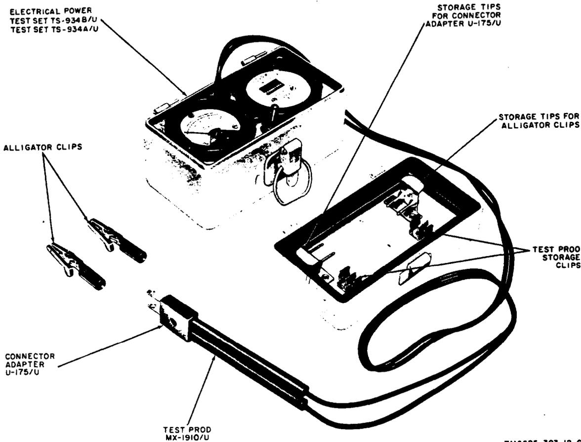
Figure 1.1. Electrical Power Test Set AN/UPM-93C only.
