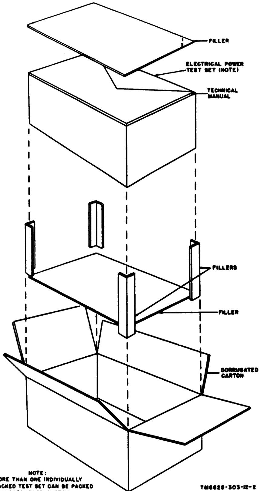
Figure 2. Typical packing.
