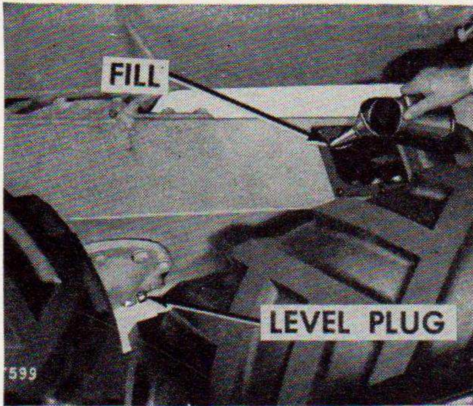
REF. 13—TANDEM DRIVE HOUSING Fill cover and level plug. Remove cover to fill or replenish housing. Keep lubricant to level of level plug hole.
