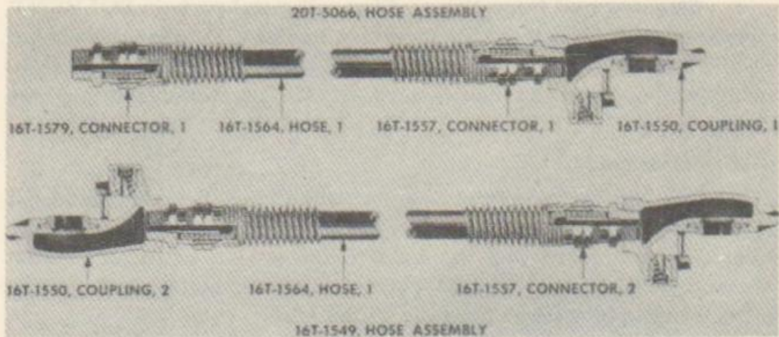
FIGURE 33. DOLLY AND SEMITRAILER AIR HOSE—SECTIONAL VIEW
