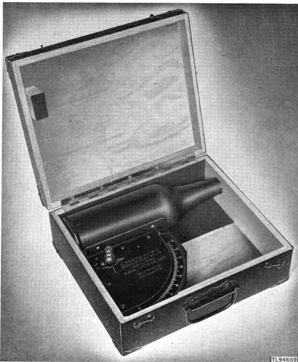
Figure 2. Clinometer in carrying case.
