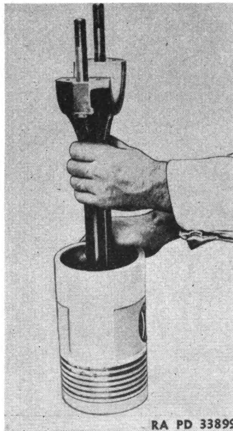
FIGURE 37.—Testing pin and bushing clearance.
