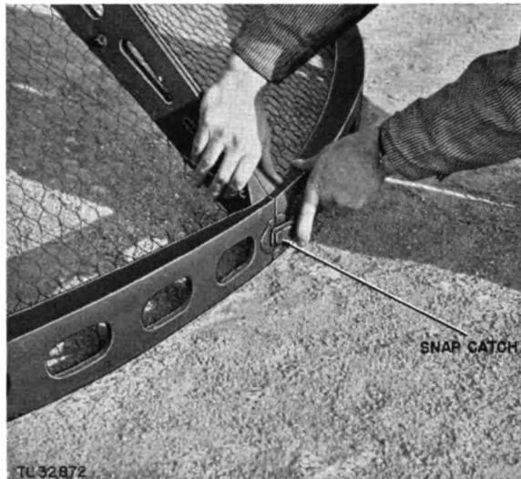
Figure 12. Tightening clamp on antenna assembly.
