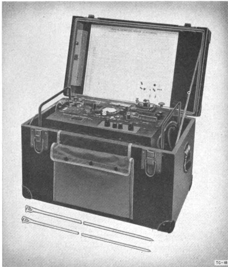
Figure 182. Repeater Set TC-19, Intermediate Telegraph Repeater.
