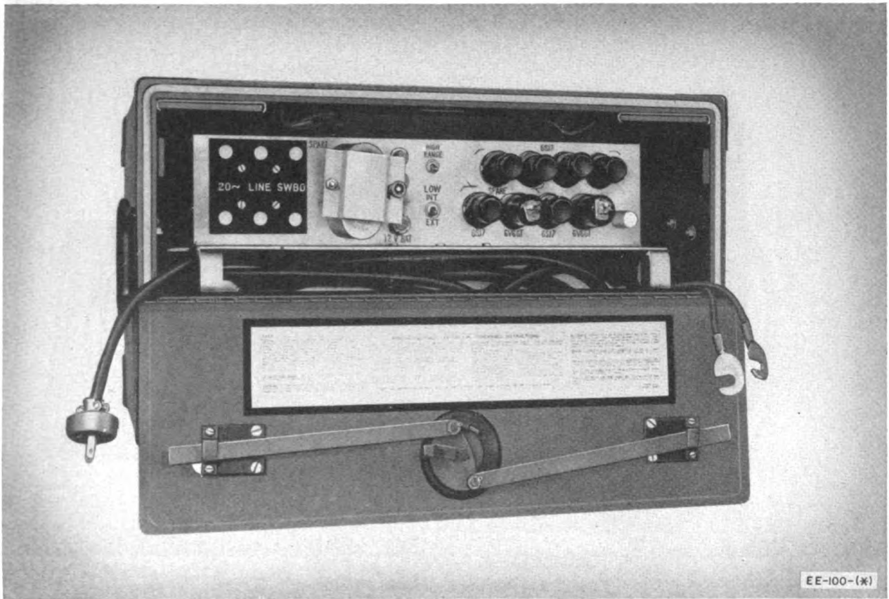
Figure 69. Ringing Equipment EE-100-(A).
