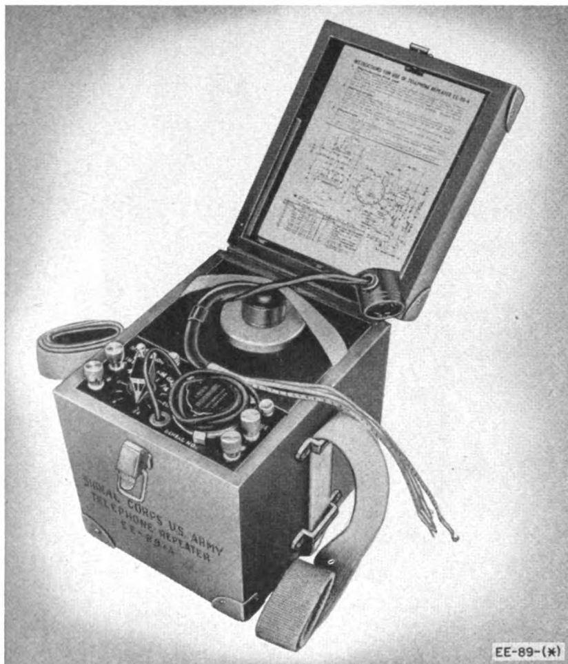
Figure 65. Telephone Repeater EE-89-A.
