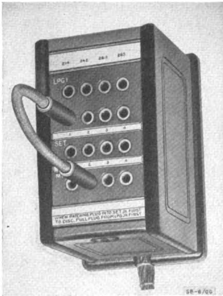
Figure 130. Telegraph Switchboard SB-6/GG.
