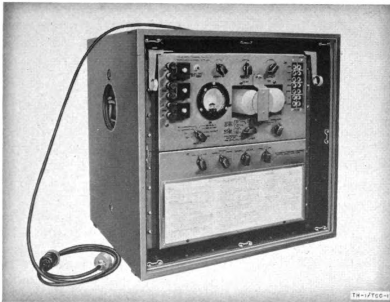
Figure 203. Telegraph Terminal TH-1/TCC-1.
