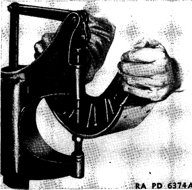
FIGURE 44.—Riveting brake lining.
