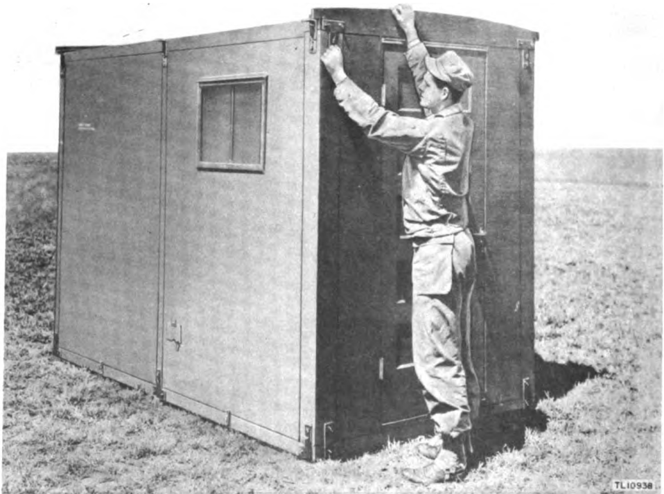
Figure 30. End roof support, installed.
