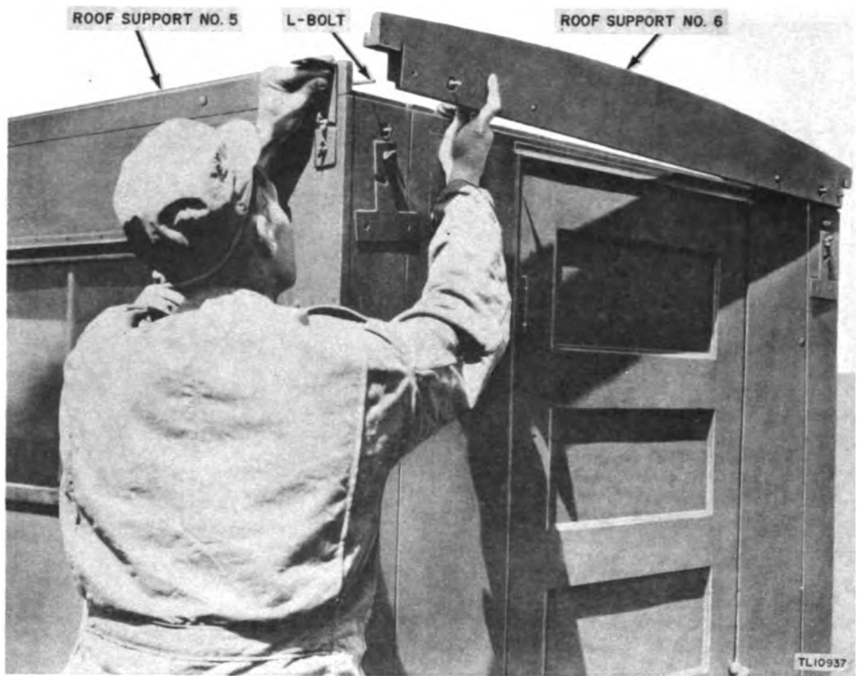
Figure 29. Installation of L-bolt in end roof support.
