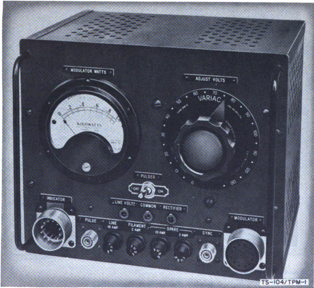
Figure 70. Test Unit TS-104/TPM-1.
