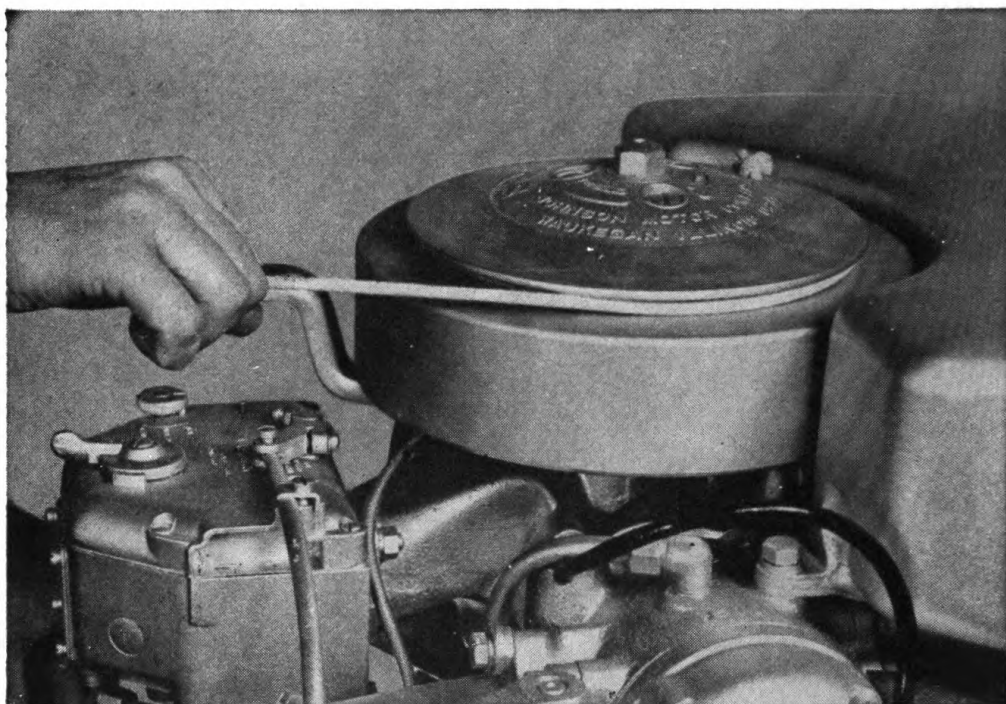
Figure 89. Pull starting cord. Grasp starting cord as shown and spin flywheel with a sustained, strong pull. Do not jerk rope.
