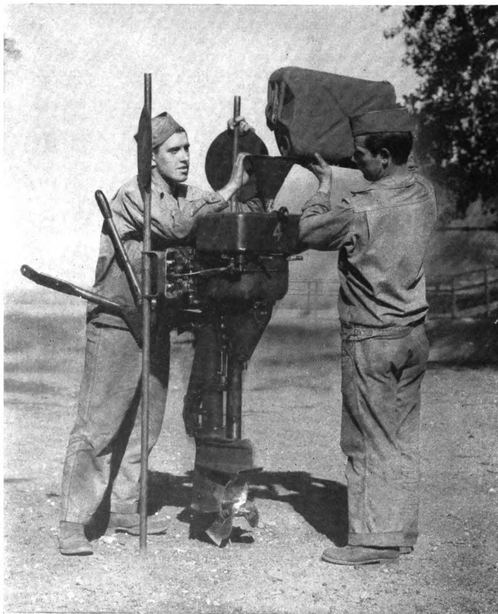
Figure 5. Pouring fuel into storm-boat motor gasoline tank.
