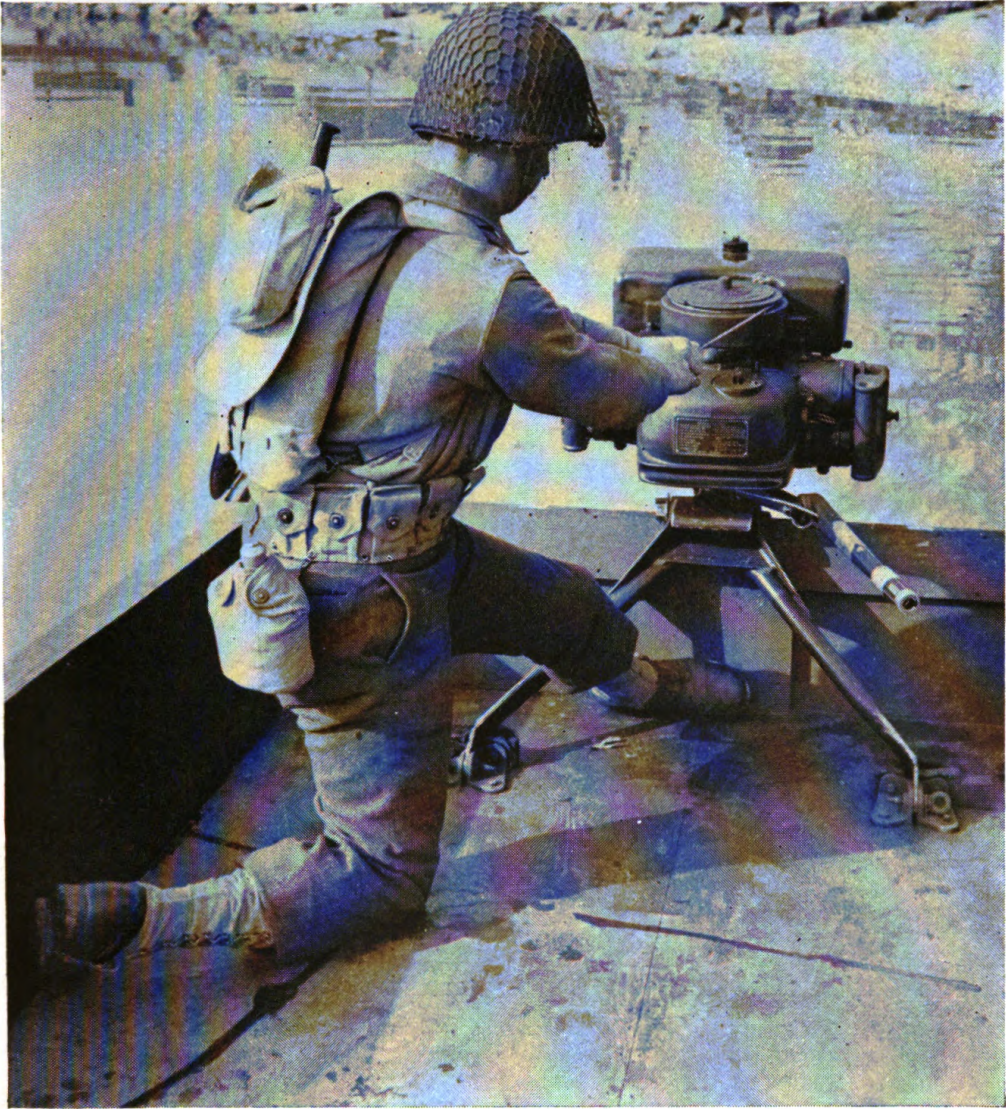
Figure 42. Spin flywheel. (Grasp starting cord as shown and spin flywheel with a sustained, strong pull. Do not jerk rope. Note operator's position.)
