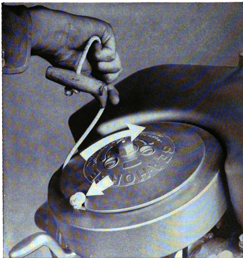
Figure 86. Wrap starting cord clockwise around starting pulley placing knot of cord in notch of drum.
