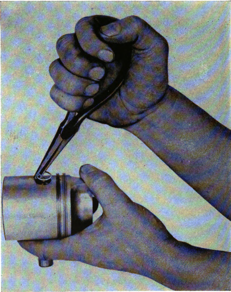
Figure 75. Installing bottom piston-pin spring ring. (Note position of hands.)
