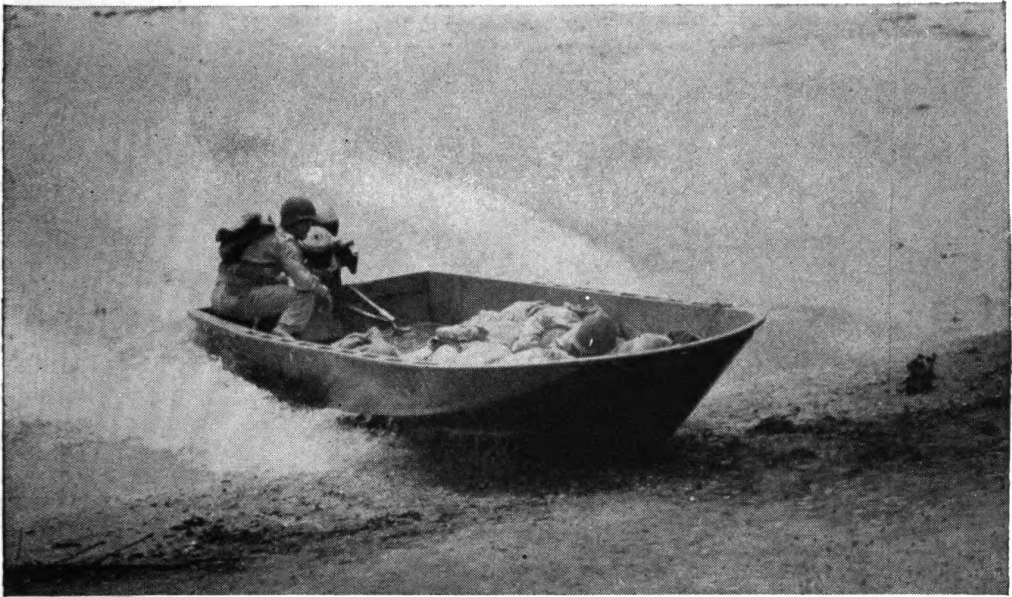
Figure 32. Beaching storm boat under power. (Note position of passengers. The operator has moved out of the way of the motor which is tilting inboard.)
