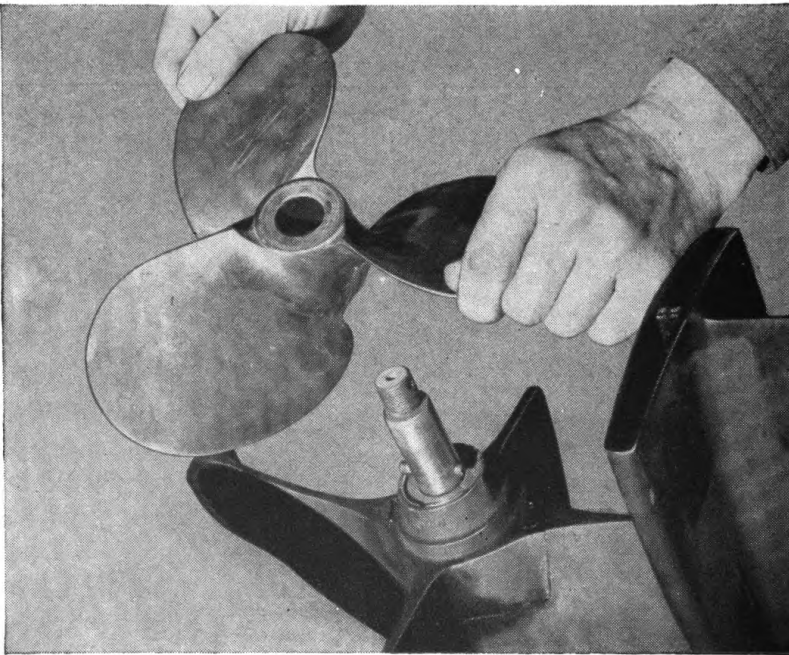
Figure 48. Remove propeller from propeller shaft
