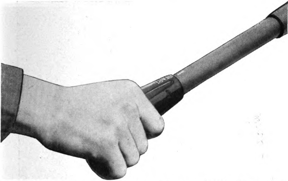
Figure 39. Set steering grip to "start" to give correct throttle adjustment for starting.
