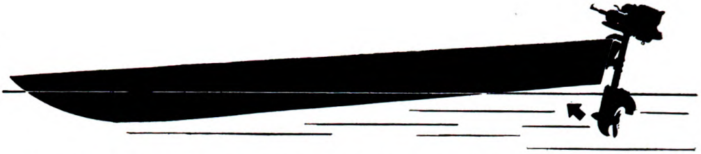
Figure 22. When propeller is tilted too close to stern, bow is low in the water.
