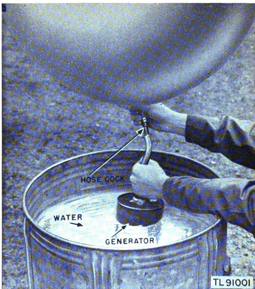
Figure 4. Hydrogen Generator ML-303/TM, in operation.
