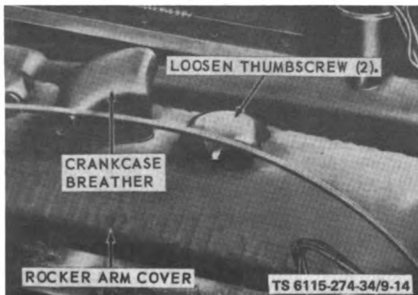
Figure 9-14. Rocker Arm Cover, Removal and Installation
