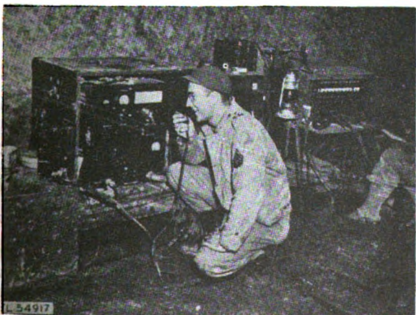
Figure 6-83. Radio Set SCR-543 and Switchboard BD-72 in operation.
