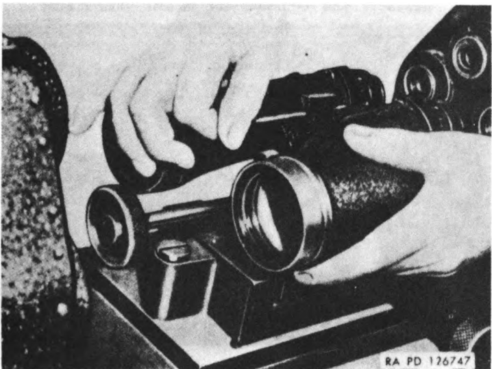
Figure 64. Installing binocular in binocular testing fixture 41-F-2987-457.
