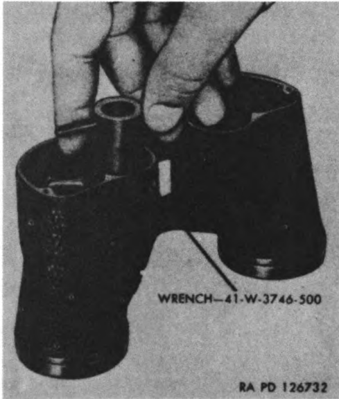
Figure 47. Removing or installing reticle adapter A185479 with wrench 41-W-3746-500.
