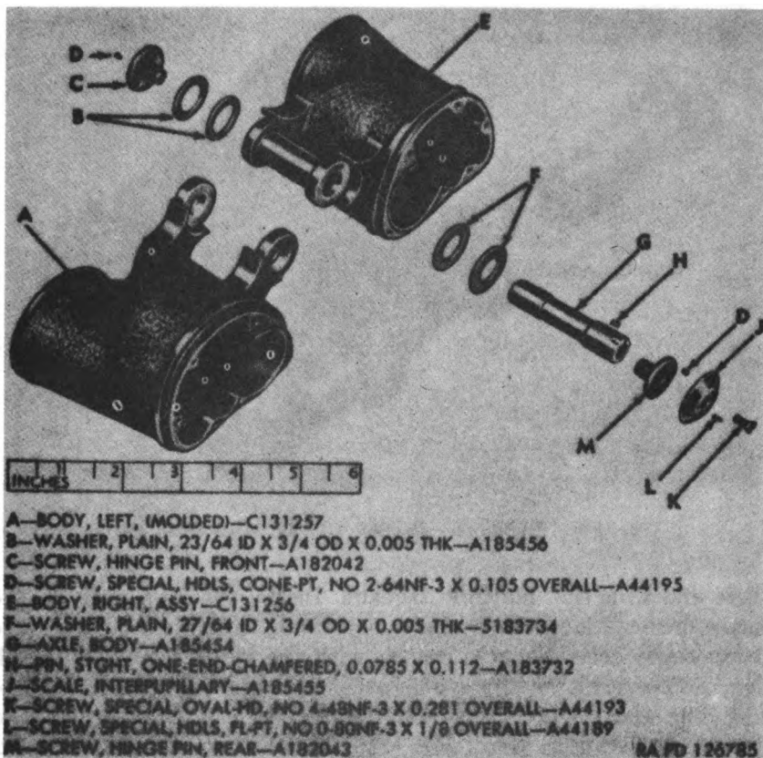
Figure 98. Body assembly C151255 — exploded view.
