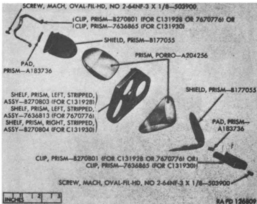
Figure 122. Prism shelf assembly C131928 or 7670776 or C131930 — exploded view.
