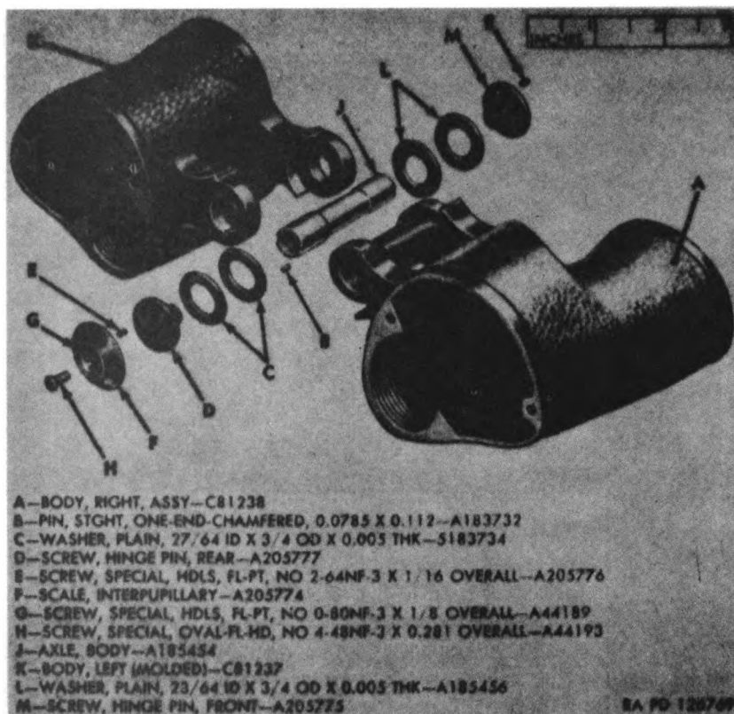
Figure 82. Body assembly C81231 — exploded view.
