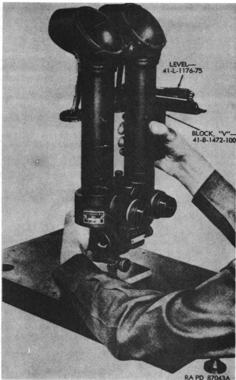
Figure 195. Bringing right telescope into true vertical position.
