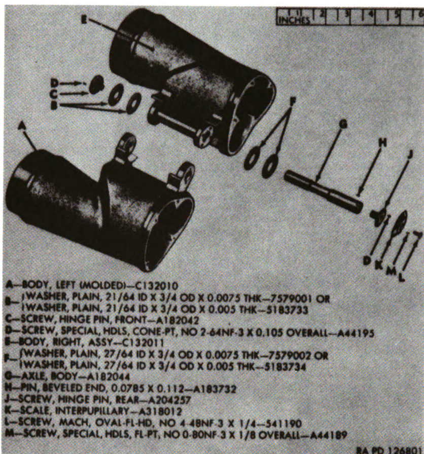
Figure 114. Body assembly C132000 — exploded view.
