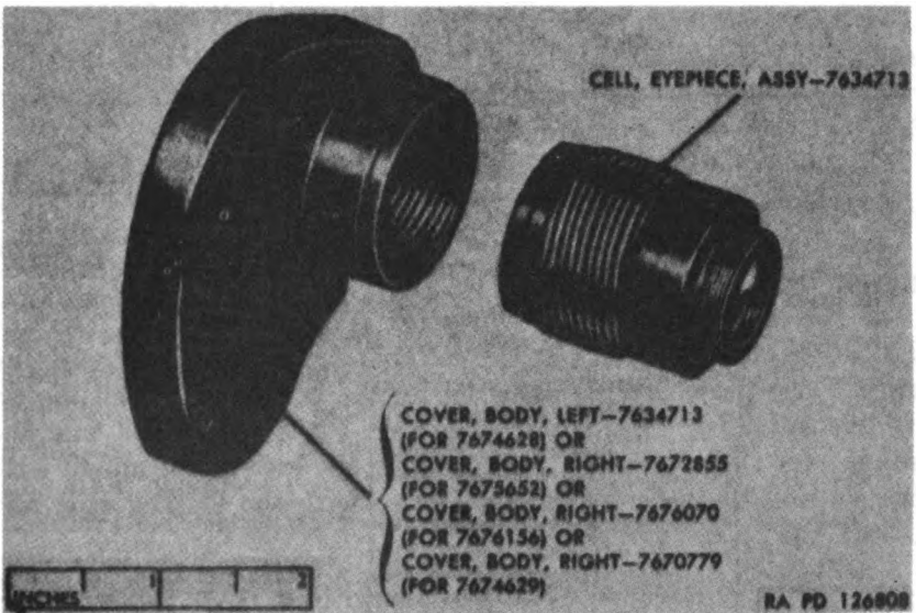
Figure 181. Body cover assembly 7674628 or 7674629 or 7675652 or 7676156 — exploded view.
