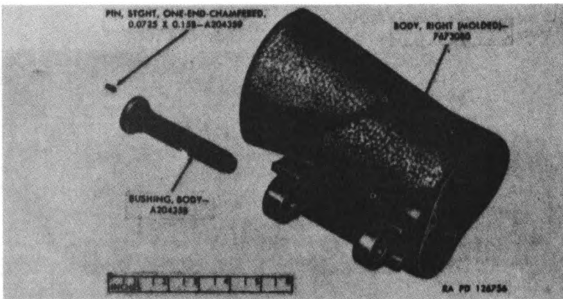
Figure 72. Right body assembly C80622 — exploded view.
