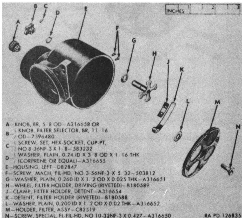
Figure 148. Left housing with filter holder assembly C82518 — exploded view.
