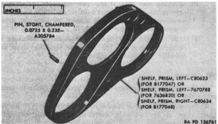
Figure 77. Stripped left prism shelf assemblies B177047 (M7 only), 7636820 (M16 only), or stripped right prism shelf assembly B177048 — exploded view.
