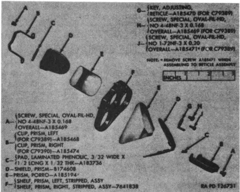
Figure 46. Prism shelf assembly — C79389 (left) or C79390 (right) — exploded view.
