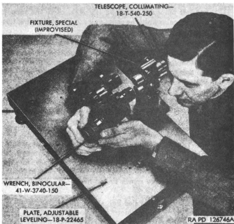
Figure 83. Rotating eccentric ring and objective cell.
