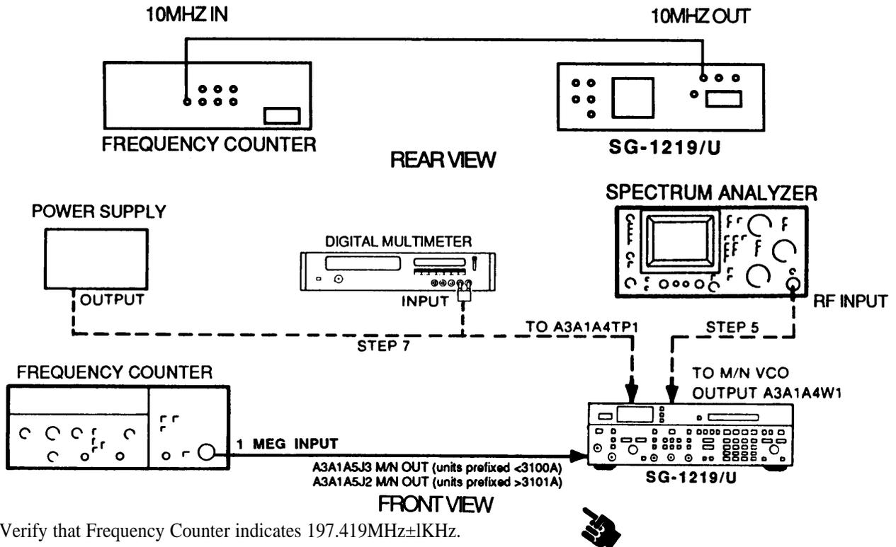
3. Verify that Frequency Counter indicates 197.419MHz±1KHz.
