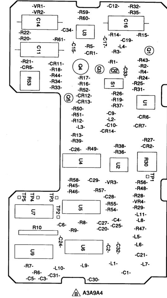
Figure FO-4. A3 Assembly Component Locator Diagram (Sheet 4 of 5). Change 2
