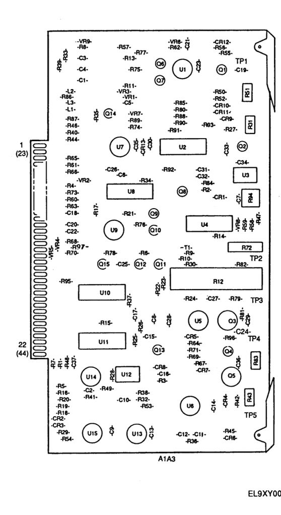
Figure FO-2. A1 Assembly Component Locator Diagram (Sheet 1 of 2).
