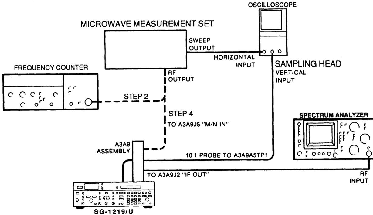
4. Connect Microwave Measurement Set RF output to A3A9J5 in place of A3W8 (white/orange).
