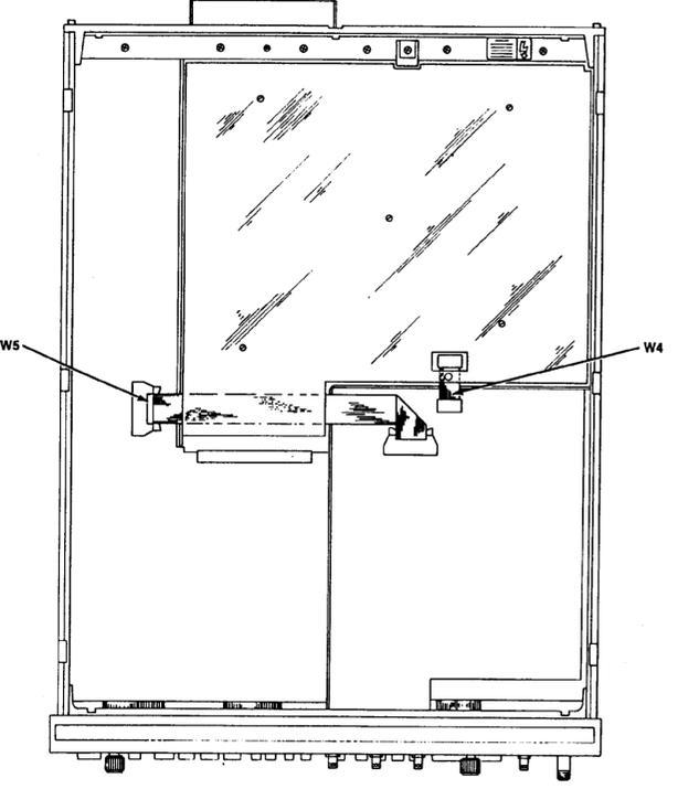
Figure FO-1. Assembly and Cable Locator Diagram (Serial Prefix <3100A>.
