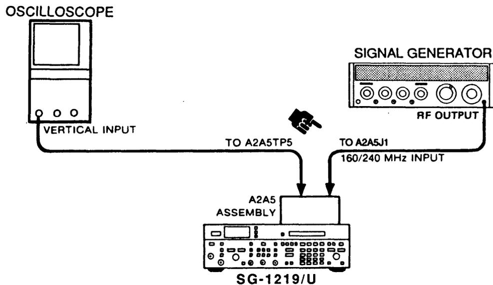
4. Observe clock signal on Oscilloscope display.
