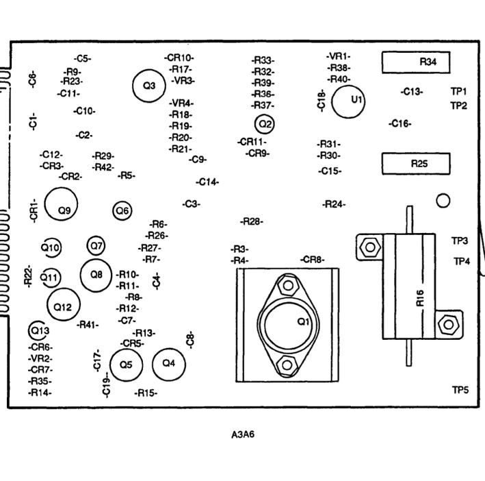
Figure FO-4. A3 Assembly Component Locator Diagram (Sheet 3 of 5).
