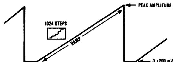
4. Adjust A2A7R34 for approximately + 10V ramp peak-to-peak and verify that ramp contains no discontinuities.
