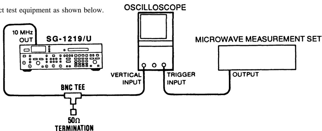
2. Set FREQ adjustment on A3A8 (fig. FO-4) so signal on Oscilloscope is not drifting.
