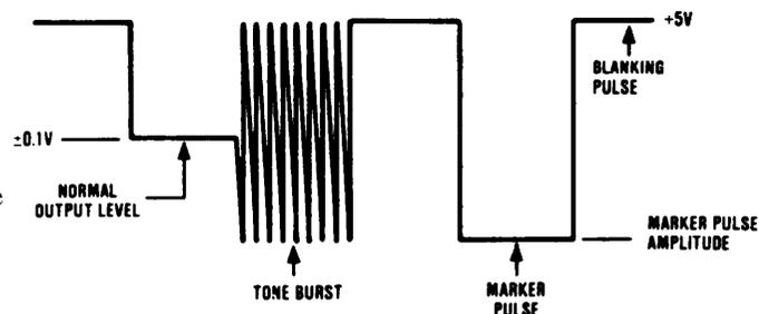
7. Adjust A2A7R50 for a marker pulse -5V below reference.
