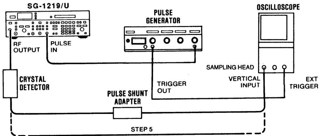
2. Set Pulse Generator for a 1 MHz pulse rate with a pulse width of 300ns and pulse height of  $\approx 5V$  5V peak. Set Variable Attenuator for 10dB attenuation.
