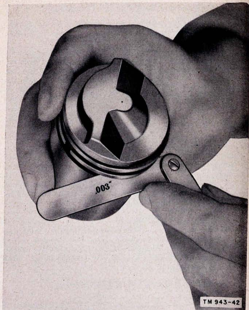
Figure 42. Checking piston ring side clearance.
