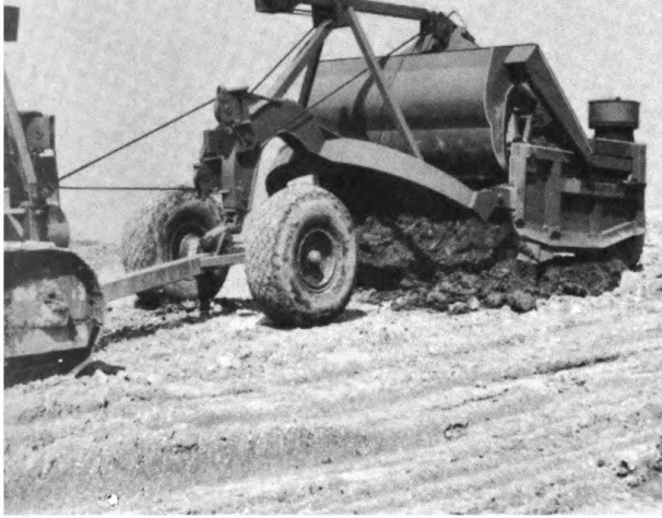
APRON RAISED TO FULL HEIGHT TO PERMIT DIRT TO FALL OUT
