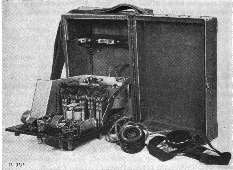
FIGURE 3.—Interior of test set EE-65.
