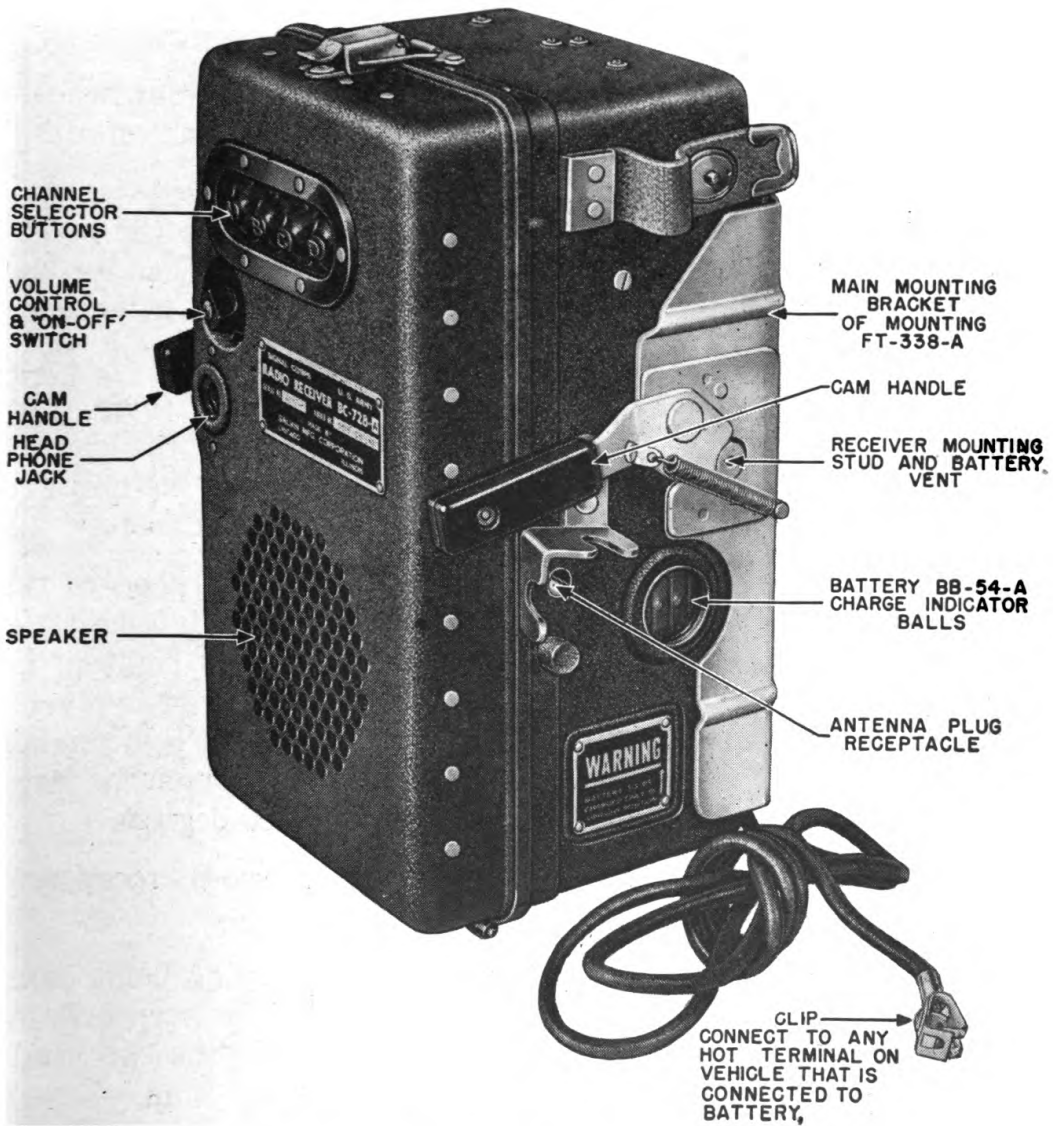
FIGURE 10—RADIO RECEIVER BC-728-A, SHOWN IN MAIN MOUNTING BRACKET OF MOUNTING FT-338-A
