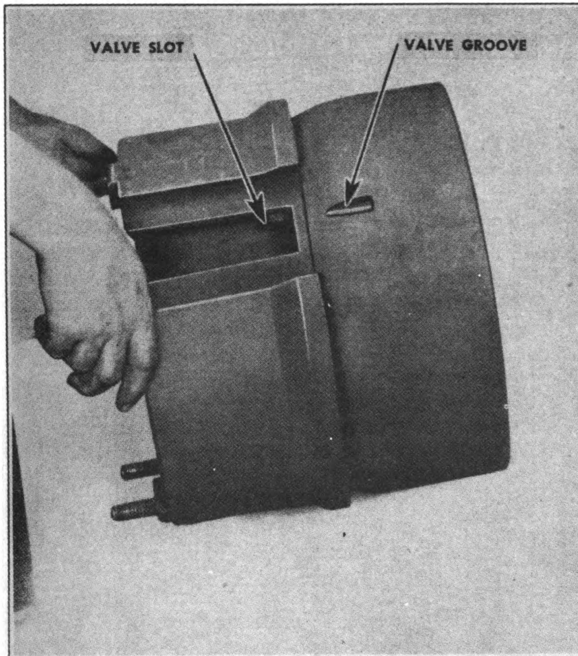
FIGURE 21. INSTALLING BRAKE DRUM—REAR
