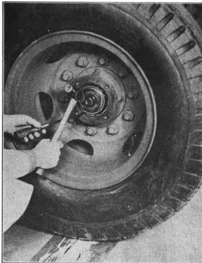
FIGURE 50. REMOVING FRONT AND REAR OUTER WHEEL ASSEMBLY and tap D-washer with a hammer. (Fig. 50). The D-washer and bearing may also be removed as the wheel assembly is pulled off.
