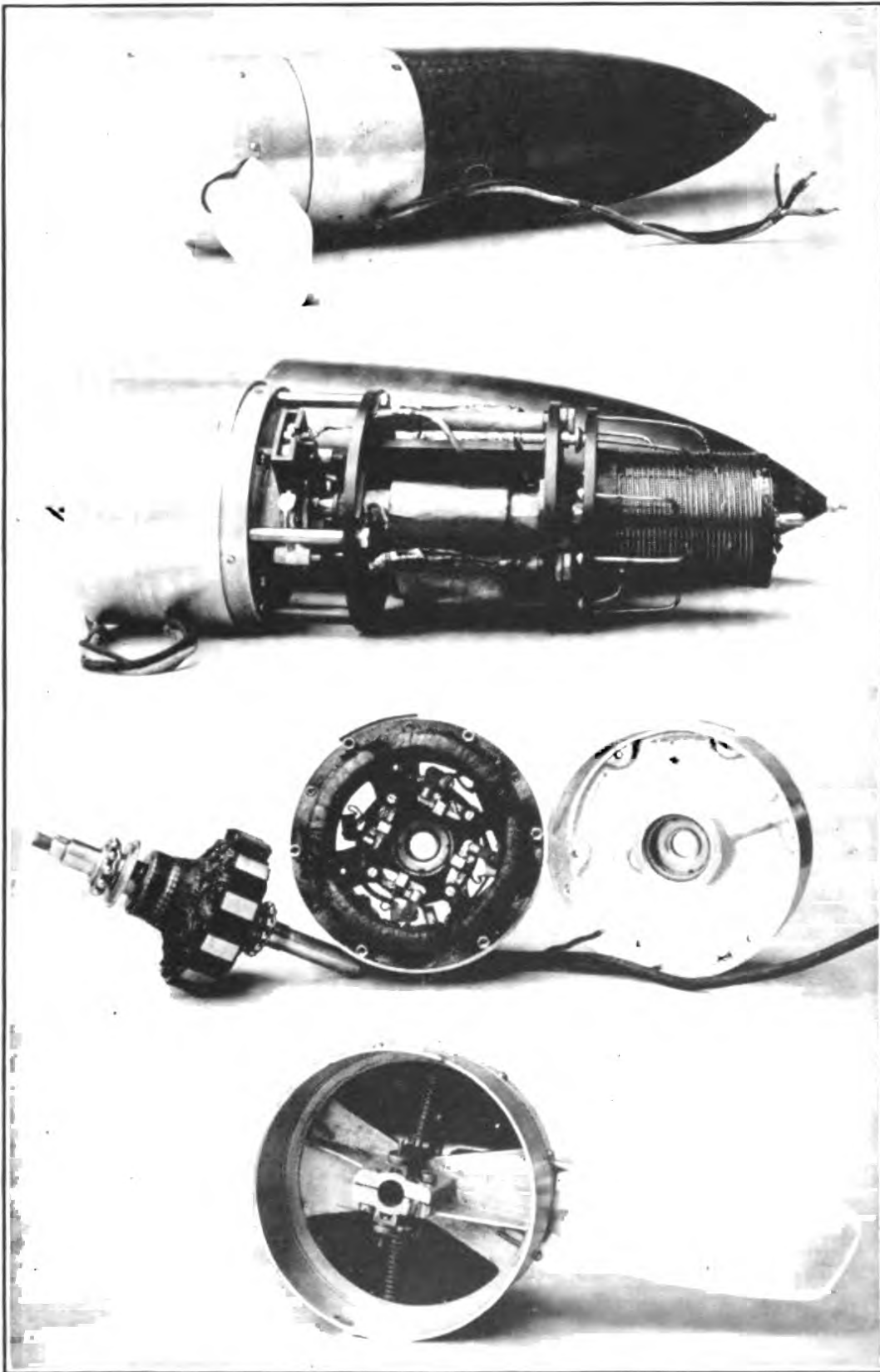
Fig. 1—Top to Bottom: Type SCR-73 Set Assembled. Casing Removed Showing Radio Apparatus. Rotor and Stator of Alternator. Airfan and Governor.
