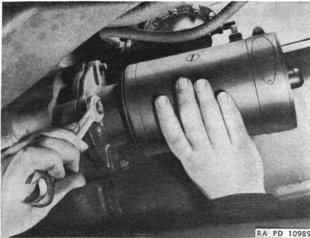
FIGURE 74.—Starting motor removal.
