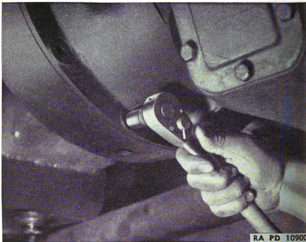
FIGURE 97. —Disconnecting engine bell housing from transmission.
