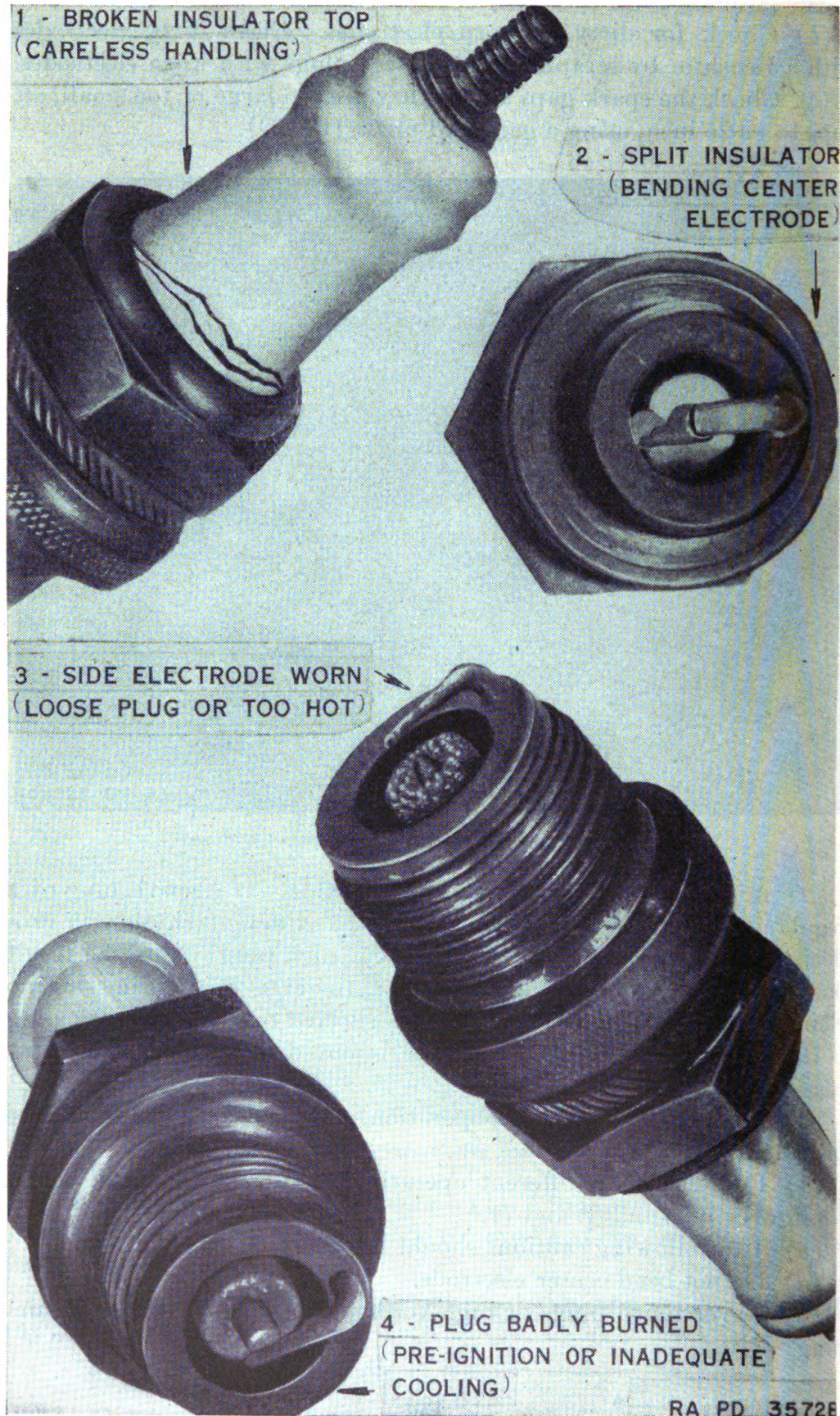
FIGURE 70①.—Effects of operating conditions on spark plugs.
