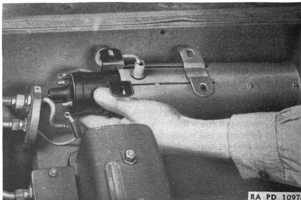
FIGURE 58.—Removing ignition coil from shielding.
