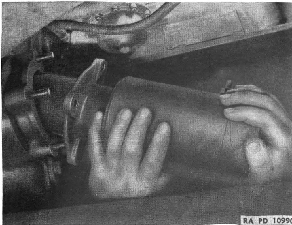
FIGURE 75.—Starting motor removal.
