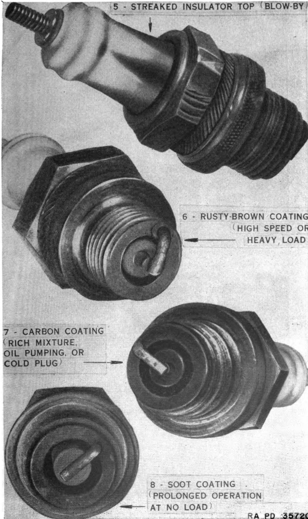
FIGURE 700.—Effects of operating conditions on spark plugs.
