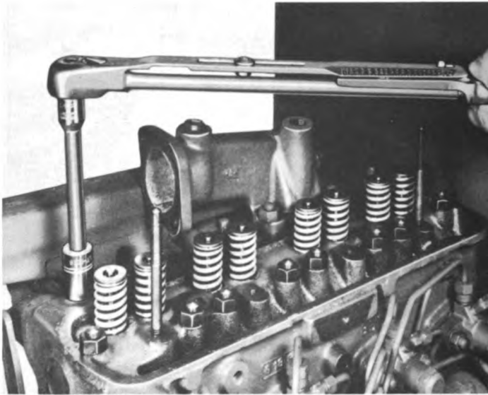
Figure 45. Tightening cylinder head stud nuts.
