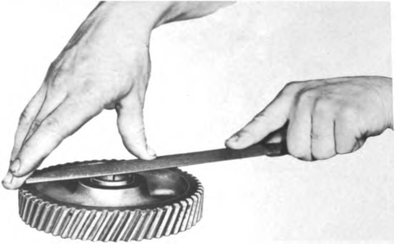
1 Prick punch marks 2 Size marks Figure 112. Correcting thrust clearance.
