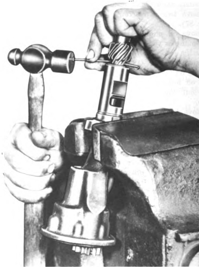
Figure 88. Removing drive gear pin from oil pump.
