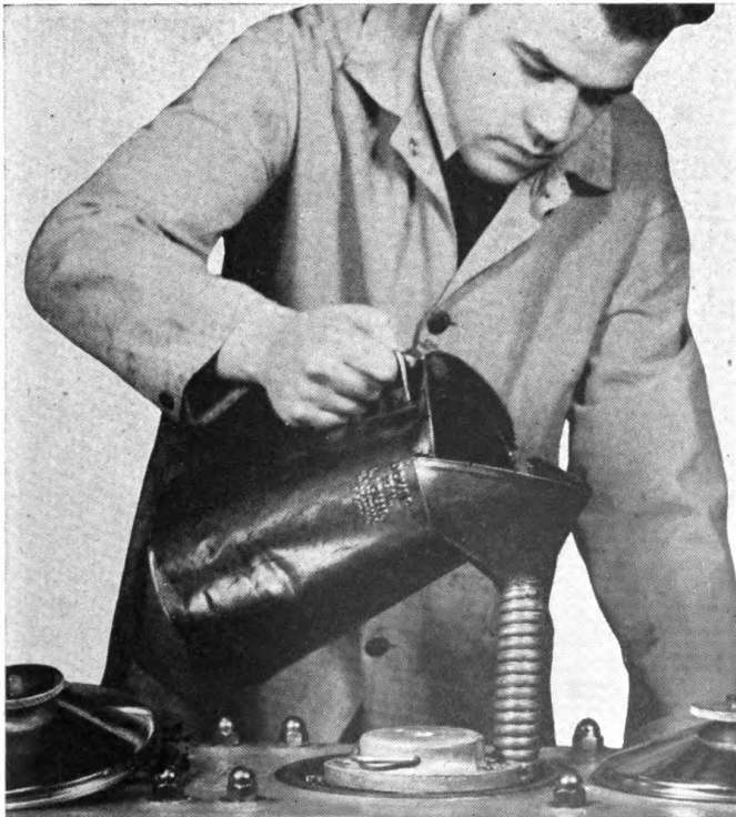
FIG. 4—Filling Engine with Oil
