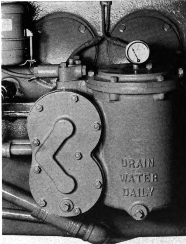
FIG. 8—Lubricating and Fuel Oil Filters
