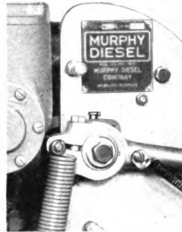
Control lever, oil every 128 hours. Use OE-10.
