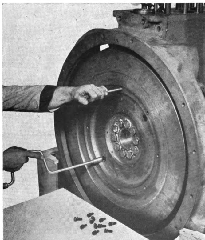
FIG. 44—Installing Capscrews to Hold Slinger in Position
