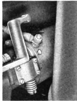
Starter bearings, oil every 512 hrs. Use OE-10.
