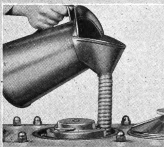
Drain at points indicated and refill through cover every 64 hours. Use OE-30 above 32° F. OE-10 below 32° F.
