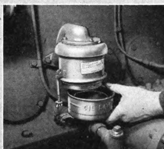
Breather Air Cleaner, empty and refill every 64 hours.
