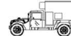
M1097 TRUCK UTIL HEAVY VARIANT HMMWV/ M1113 EXP CAP HMMWV W/RIGID WALL SHELTER
